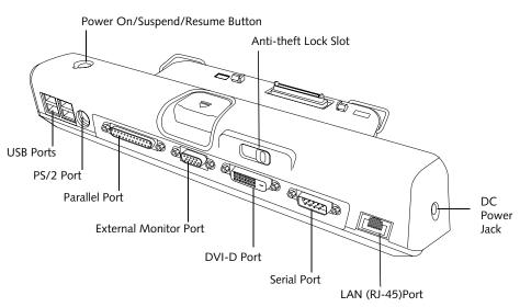
Figure 4-11. Port Replicator back panel
